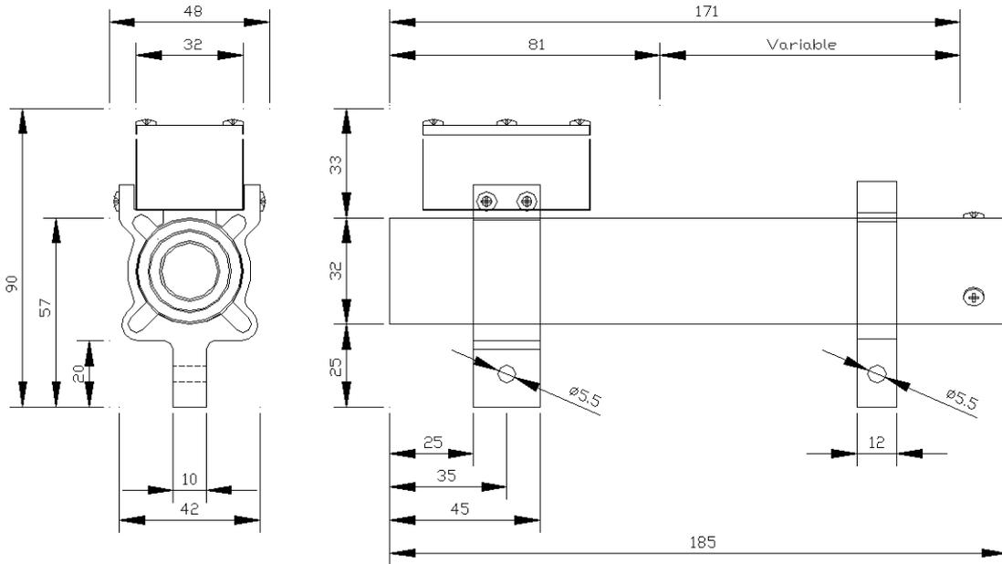
Fig. 6-5: Inboard ACP Sensor
