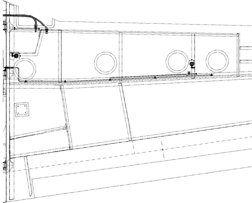
Fig. 6-3: Position of Sensors in Aircraft wing (top view)
