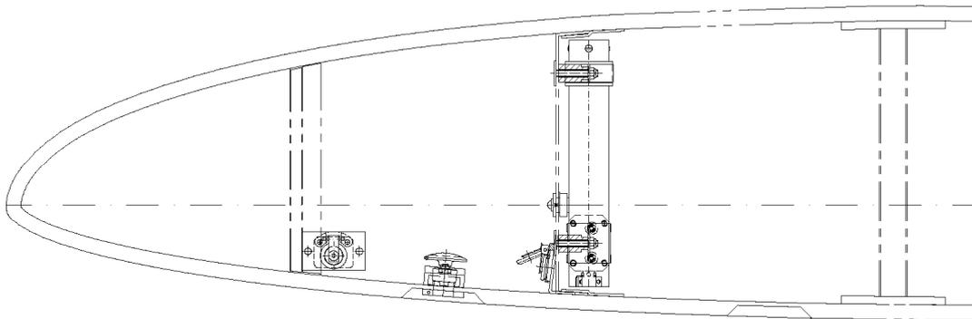
Fig. 6-4: Position of Sensors in Aircraft wing (wing section)
